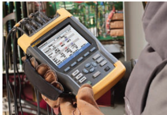
Fluke 435 Three-Phase Power Quality Analyser
