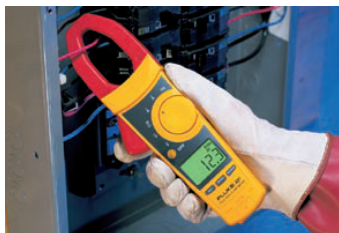
Fluke 337 True-rms Clamp Meter
