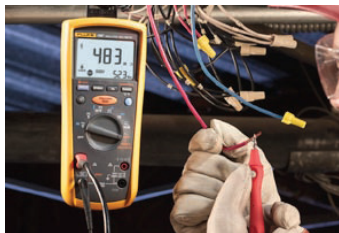
Fluke 1587 Insulation Multimeter
